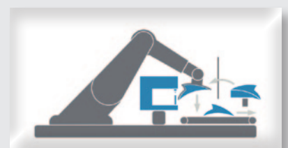
- 3D Robot cell (stationary sewing head) - Tool/workpiece: robot-guided
