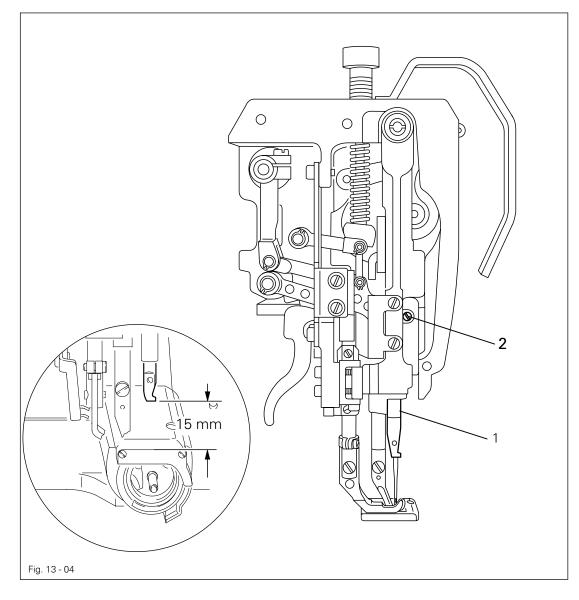
• Adjust the needle bar 1 (screw 2) without twisting according to the rule.
